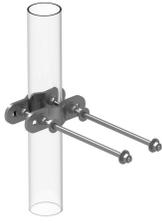
PIM-Guard® Round Member Cable Support Bracket for Block Hangers - Two 3/8" threaded rods for up to 12 hangers. Install with torque wrench set at 10 to 15 ft-lb to meet carrier PIM requirements.
