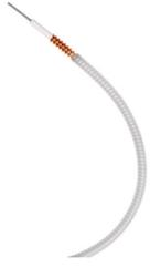
PTS1-50, HELIAX® Superflexible High Power, High Temperature 50 Ohm Plenum Rated Coaxial Cable, corrugated copper, 1/4 in, white FR-PVC jacket.
