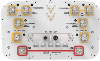
10-port sector/multi beam antenna, 2x 698-960 sector and 8x 1710-2690 multi beam, 65° sector and 33° 4x multi beam, 5x RET with tilt indicators
