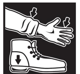
Wear shoes with rubber soles and heels. Wear protective clothing including a long-sleeved shirt and rubber gloves.
