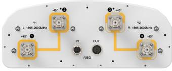
4-port sector antenna, 4x 1695–2690 MHz, 65° HPBW, 1x RET . The two high band arrays utilize a common tilt.
