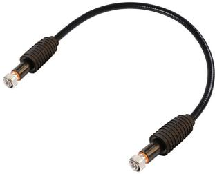
HELIAX® 1/2" SureFlex® Fire retardant Jumper with interface types 4.3-10 Male and 4.3-10 Male with HELIAX® SureGuard weatherproofing, with black non-halogenated fire retardant polyolefin jacket B2ca-S1a-d1-a1
