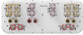
16- Port sector antenna, 4x 698-896, 8x 1695-2360 and 4x 3550-3700MHz, 65° HPBW, 3x RETs and 3x SBTs
