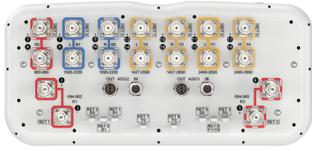
18-port sector antenna, 2x 694–862, 2x 880–960, 2x 694–960, 4x 1427–2690, 4x 1695–2200 and 4x 2490–2690 MHz, 65° HPBW, 8x RET
