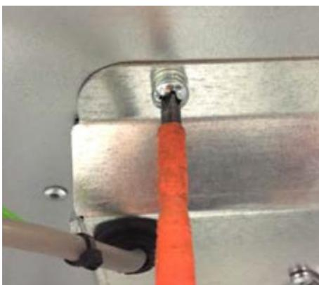
Figure 13: Removing Fan Module 1
