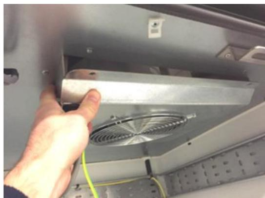
Figure 14: Removing Fan Module 2
