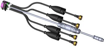
HELIAX® M-LOC Multiport cluster 5 ports SureFlex® cable assembly with interface type M-LOC latching male to 4.3-10 male with HELIAX® SureGuard weatherproofing, with AISG converter in the center port, size 1/4", length 0.45 meters
