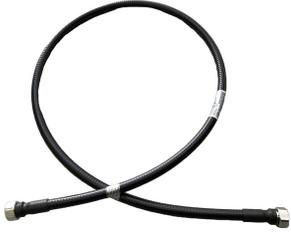
HELIAX® 1/2" Superflexible Fire retardant SureFlex® Jumper with interface types 7-16 DIN Male and 7-16 DIN Male,, with black nonhalogenated fire retardant polyolefin jacket B2ca-S1a-d1-a1
