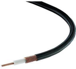
FSJ4RK-50B, HELIAX® Superflexible Foam Coaxial Cable, corrugated copper, 1/2 in, black non-halogenated, fire retardant polyolefin jacket B2ca-s1a-d1-a1 (CPR testing is conducted annually please reference the website for latest classification)
