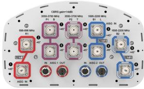
10-port sector antenna, 2x 698–896, 4x 1695–2200 and 4x 3550–3700 MHz, 65° HPBW, 2x RETs and 2x SBTs
