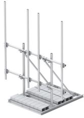
High Capacity Non-Penetrating Roof Frame, 10 ft face, Four 2-7/8 in OD x 126 in pipes
