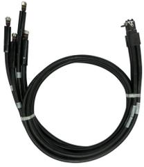
HELIAX® M-LOC Multiport cluster 4 ports SureFlex® cable assembly with interface type M-LOC latching male to 4.3-10 male, size 3/8", length 3 meters, covered by conduit shield
