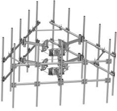
Heavy Duty Double T-Arm Monopole Mount, Includes (2) Ring Mounts for 15"-50" OD Monopole, 14.5 ft x 3-1/2" OD face pipes, (12) 2-7/8" OD x 120" Antenna Pipes
