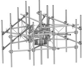
G23RHDX Monopole Sector Frame with spine extension for RRU Mounting, 12.5 ft x 2.88 in OD face pipes, includes twelve 2.88 OD x 96 in antenna pipes
