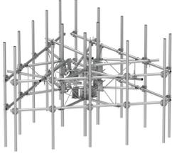
G23RHDX Monopole Sector Frame with spine extension for RRU Mounting, 14.5 ft x 2.88 in OD face pipes, includes fifteen 2.88 OD x 120 in antenna pipes
