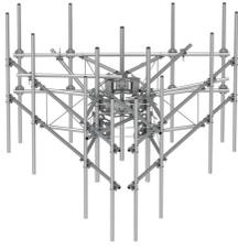
G23RHDX Monopole Sector Frame with spine extension for RRU Mounting, 14.5 ft x 2.88 in OD face pipes, includes fifteen 2.88 OD x 96 in antenna pipes
