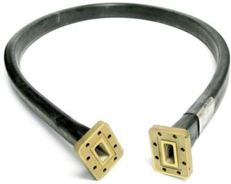
FlexTwist® Flexible Twist for WR42, 17.7–26.5 GHz, with interface types PBR220 and PBR220, 300 mm
