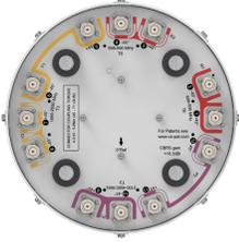
12-port quasi-omni antenna, 4x 698-896, 4x1695-2690 and 4x 3100-4000MHz, 360° horizontal beamwidth, Fixed tilt.
