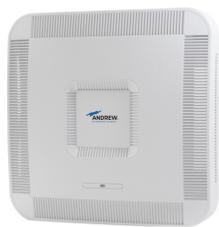
Carrier Access Point with MIMO 2x2 Radio Module for Low Power APT 700, EDD 800, CEL 900, DCS 1800 and IMT 2100 Applications, Copper fed, PoE++
