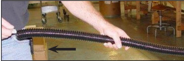
Remove electrical tape from the trunk cable and corrugated protection tube. While holding the protection tube straight pull the tube away from cable.
