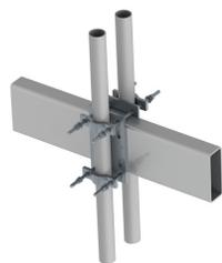
XP-PM Dual RRU Mount Bracket Kit for Back-to-Back Mounting of (2) RRUs to 3.5-4.5" Square or 3-6" Rectangular Tube. 2-3/8" to 3-1/2" OD Mount Pipes ordered separately.
