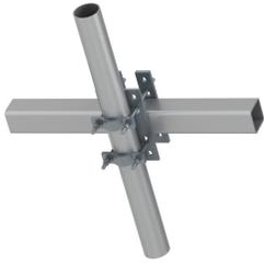
XP-PM RRU Mount Bracket Kit for Mounting of (1) RRU to 3.5-4.5" Square or 3-6" Rectangular Tube. 2-3/8" to 3-1/2" OD Mount Pipes ordered separately.
