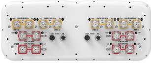
16-port, low band diplexed antenna, 4 x 698-798 MHz, 4 x 824-894 MHz and 8 x 1695-2360 MHz, 65° HPBW, 6 x RET
