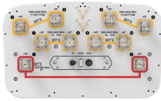
10-port sector/multibeam antenna, 2x 694–960 sector and 8x 1695–2400 multibeam, 65° sector and 33° 4x multibeam, 3x RET
