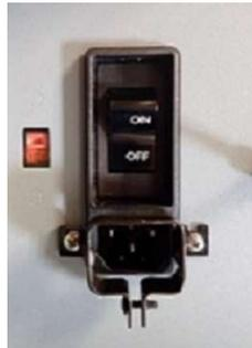
22. Remove the “Jumper” from the dehydrator that was installed in step 8. **The MT050C requires the tank to be completely drained before the initial power up.** Turn the power back on paying attention to the initial screen to verify that the firmware has changed to v3.0.
