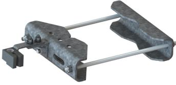
Clamping guide to protect wire cable. Clamps on to: -1.5"-8" for round members -8" for 60 degree angle -6" for 90 degree angle
