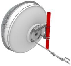
1.8m | 6ft ValuLine® Low Wind Load Antenna, dual-polarized, 7.125 – 8.500 GHz, white, PDR84 flange
