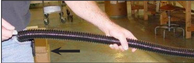
While holding the protection tube straight pull the tube away from cable.
