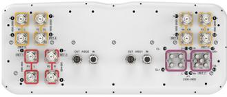
20-port sector antenna, 4x 694-960 (R1-R2), 8x 1695-2690 MHz (Y1-Y4) 65° HPBW and 8x 2300-3800 MHz (P1), 90° HPBW Beamformer, 7x RET
