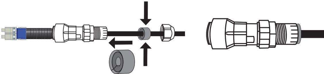
Wrap the rubber split grommet around the jacketing with the stepped end towards shroud body. Push gasket into the clamping tyres. Approximately 0.9 mm will protrude from the tyres when fully installed.
