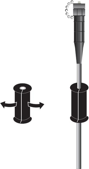
**2** Place the hanger over the grommet and place in support structure.
