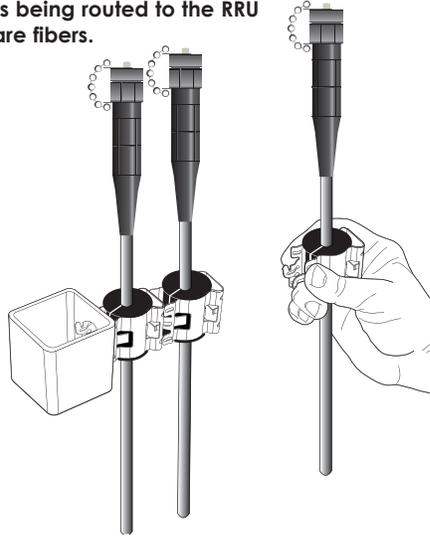
**Connectors are fully weather sealed and do not require additional weatherizing. Unused power conductors should be left with the protective cap in place.**
