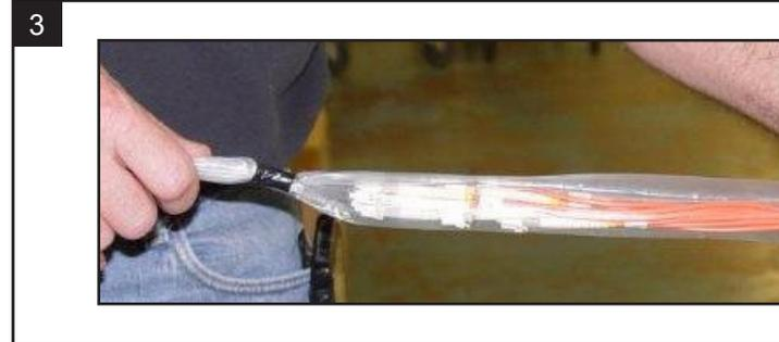
3 After you have pulled the fiber and power conductors remove electrical tape from the trunk cable and remove clear tube for access to all optical connectors.
