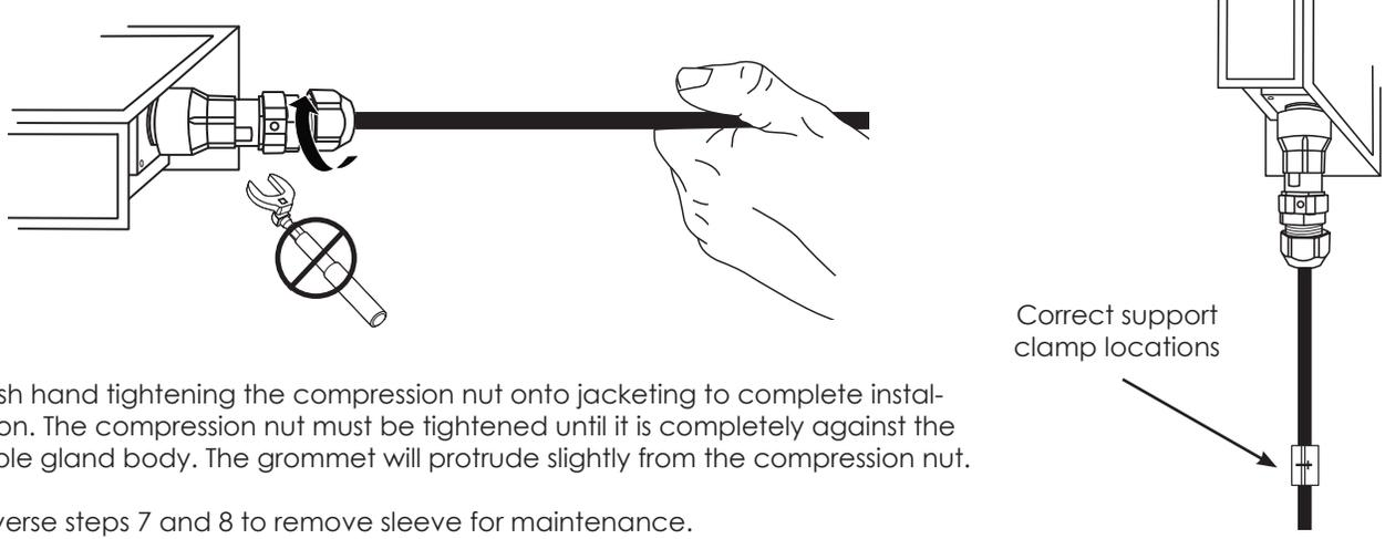
Finish hand tightening the compression nut onto jacketing to complete installation. The compression nut must be tightened until it is completely against the cable gland body. The grommet will protrude slightly from the compression nut.
