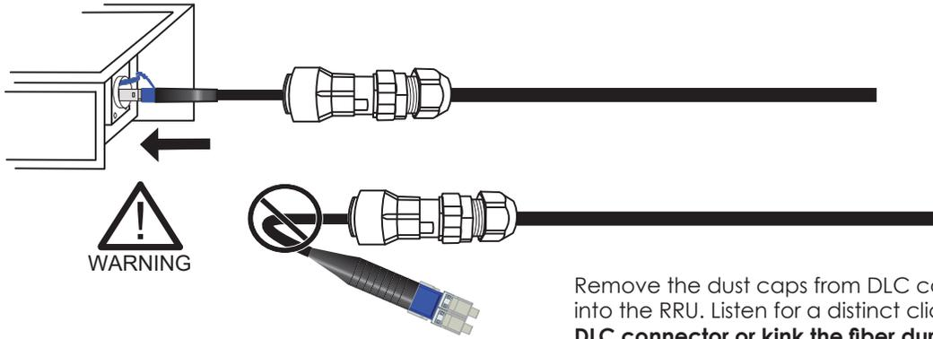
Remove the dust caps from DLC connector and seat into the RRU. Listen for a distinct click. **Do not twist DLC connector or kink the fiber during installation.**
