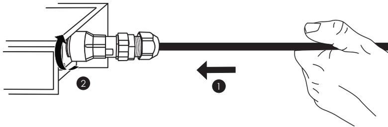
Slide the weather shroud up to the RRU. ❶ Turn top nut clockwise to secure to RRU bulkhead connector. ❷
