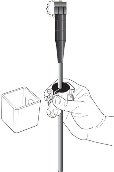
**3** Stack hangers as required. Repeat with tails being routed to the RRU and spare fibers.
