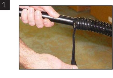
1 Remove electrical tape from the trunk cable and corrugated protection tube
