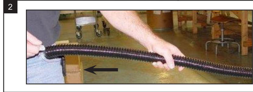
2 While holding the protection tube straight pull the tube away from cable.
