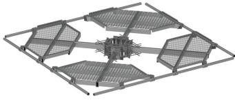
Atlas 4-Sector Monopole Platform Base kit, 15 in to 45 in OD, 2-7/8 in OD x 14 ft 6 in face. Top rail & antenna pipe/mounts ordered separately.
