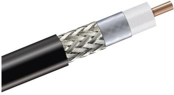
CNT-400-FR, CNT® 50 Ohm Braided Coaxial Cable, black non-halogenated, fire retardant polyolefin jacket, Dca s2 d2 Compliant
