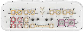
24-port sector/multibeam antenna, 4x 694–960, 4x 1695–2690MHz 65° HPBW, 8x 1710–2690MHz 4x33° HPBW and 8x 2300–3800MHz, 90° HPBW 9x RET
