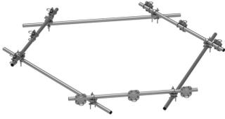
T-Arm Upgrade/Reinforcement Kit for 14' Face, 3- Sector, 2-3/8" OD x 174", with Hardware for mounting to (12) 2-3/8" Antenna Pipes
