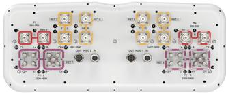
28-port sector antenna, 4 x 694-960 MHz (R1,R2), 4 x 1695-2690 MHz (Y1,Y4) and 4 x 1427-2690 MHz (Y2,Y3), 65° HPBW, 16 x 2300-3800 MHz (P1,P2), 90° HPBW, 8 x RET
