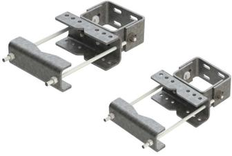
Tapered Pipe Mount Leveling Kit, attaches up to 8" OD or 60 degree angle Tower Legs, For Pipes 2-3/8" to 4-1/2" OD, U-Bolts sold separately
