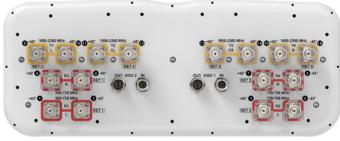
16-port, low band diplexed antenna, 4 x 698-728 MHz, 4 x 758-798 MHz and 8 x 1695-2360 MHz, 65° HPBW, 6 x RET
