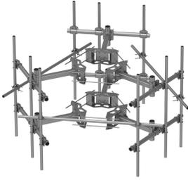
Three-Sector Double T-Arm Monopole Mount, Includes (2) Ring Mounts for 15"-50" OD Monopole, 6 ft x 3-1/2" OD face pipes, (9) 2-3/8" OD x 96" Antenna Pipes
