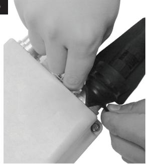
Grip the tabs on the top of boot and use to pull the boot over the coupling nut (and adapter if installed).
