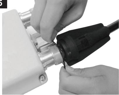
Re-position hands on wider portion of ribs, pulling outward on the ribs slide the boot into a position where it's contacting the face of the coupling nut.
