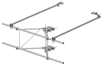
G22HD High Capacity Sector Frame with 2 7/8in OD x 14.5ft face. Base Kit Only. No antenna pipes.
