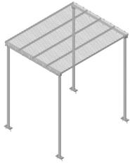
Ice Canopy, 10 ft x 15 ft, four 10 ft 6 in base shoe pipes
