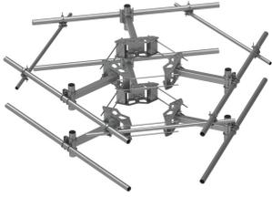
Heavy Duty Double T-Arm Monopole Mount Base Kit, Includes (2) Ring Mounts for 15"-50" OD Monopole, 12.5 ft x 3-1/2" OD face pipes. Antenna Pipes not included.
