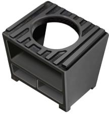
PIM-Guard®, Single-Way Snap-in Stand-off Adapter has a two slots for round member attachment. It includes one 3/4" hole for Snap-in hangers, supporting three stacks for 4-17mm or two stacks for 26-40mm cables
