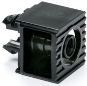
PIM-Guard® Multifunction Adapter that threads into 3/8" & 1/2" bolts & U-bolts or snaps into 3/4" holes. One 3/4" hole for Snap-in style hangers, supporting three stacks for 4-17mm or two stacks for 26-40mm cables
