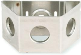
Three-Way Snap-in Stand-off Adapter has two slots for round member attachment and 3/8" holes for angle adapter integration. It includes three 3/4" holes for Snap-in hangers
