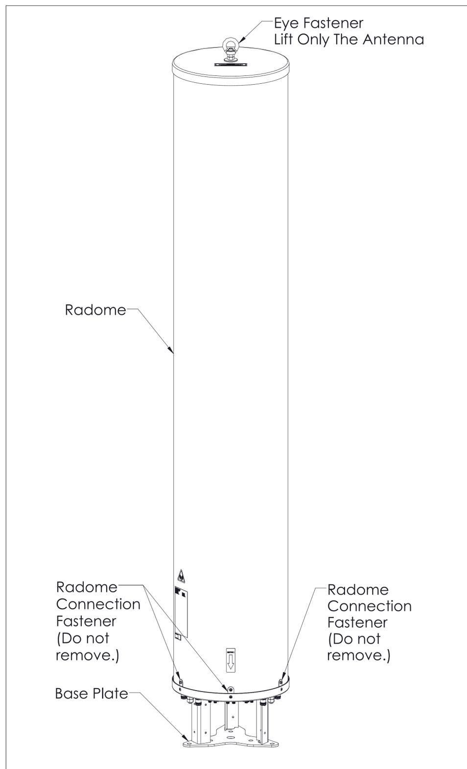
Figure 1. DIA 370mm Tri-sector antenna
