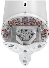
42-port tri-sector antenna, 6x617-960, 12x1695-2690MHz, 65°HPBW, 24x3300-3800MHz Beamformer, 12x RET
